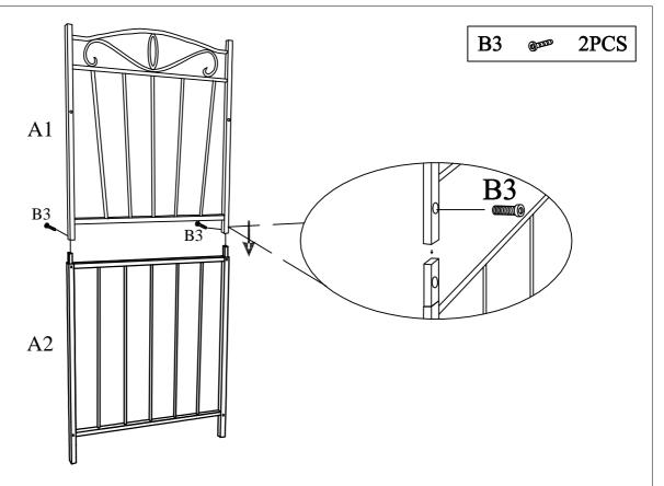
Insert Upper Back Frame A1 to Lower Back Frame A2 using Bolts B3.
