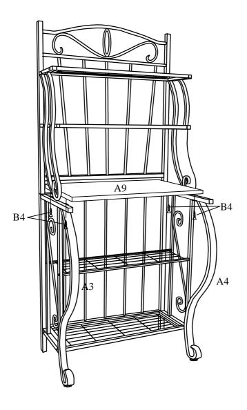
Assemble Center Panel A9 to Legs A3&A4 using Screws B4. Please tighten all Bolts B1&B2&B3 at this point.
