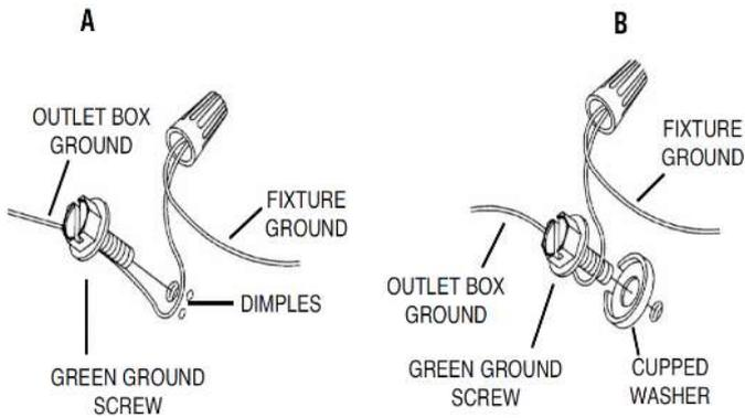
**Connect wires according to below chart**
