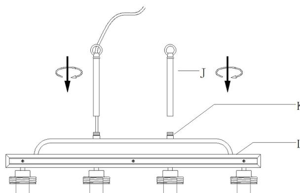
5. Attach the quick links(J)to connect the chains(I) and the loops(L) of the canopy (G)and tubes (J)
