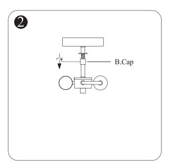
3. Attach Shade C to Light Assembly A by inserting the cut-out of the center shade washer to the threaded tubing and tighten it by screw Cap B up.
