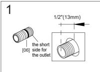
Connect to 1/2" IPS supply line. The pipe should extend 1/2" past the finished wall surface. Using the Connector [06] if needed. WARNING: Connect to Cold Water Only.
