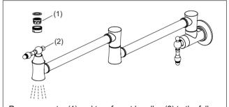
Remove aerator (1) and turn faucet handles (2) to the full on position. Turn on cold water supply and flush water line for one minute.
