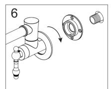
Place Flange [02] onto the faucet as shown. Thread faucet onto pipe. Tighten securely, but do not over tighten.
