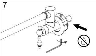
Tighten Hex Screw [07] in Anchor [04]. Slide Flange [02] over the wall Anchor [04]. Check all connections at arrows for leaks.Retighten if necessary,but do not overtighten.
