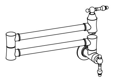
**NOTE:** THIS FAUCET IS DESIGNED TO BE INSTALLED THRU 1 HOLE,  $\Phi$ 1-3/8" MIN.
