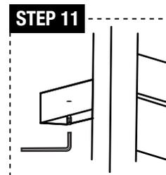
**STEP 11:** As shown in the picture, install the set screws (c) into the hole of all the tubes (a and b) using the allen wrench; fix the tube (a) onto the mounting bracket (g and h).
