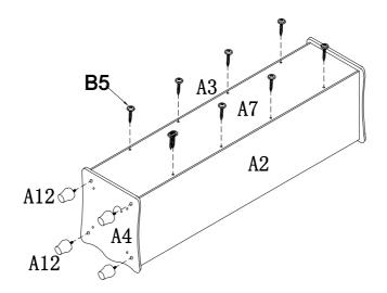
Tighten Back Panel (A7) to Side Panels (A2&A3) using Screws (B5). Attach Legs (A12) to the bottom of Bottom Panel (A4).
