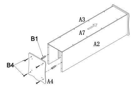
Insert Back Panel (A7) into grooves on back of Side Panels (A2&A3) and Top Panel (A1). Then assemble Bottom Panel (A4) to Side Panels (A2&A3) using Wood Dowels (B1) and Screws (B4).
