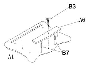
Assemble Top Divider (A6) to Top Panel (A1) using Wood Dowels (B7) and Screws (B3).
