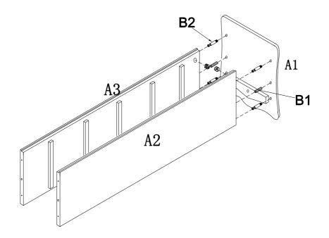
Assemble Top Panel (A1) to Side Panels (A2&A3) using Cam-Bolts (B2) and Cam-Locks(B2), Wood Dowels (B1).
