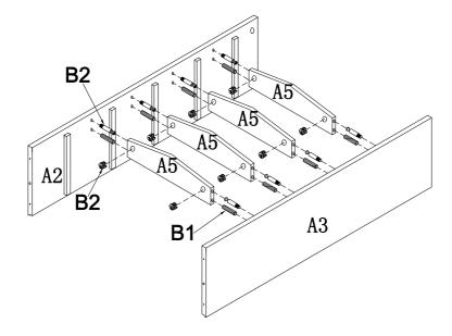
Assemble Dividers (A5) to Side Panels (A2&A3) using Wood Dowels (B1), Cam-bolts (B2) and Cam-locks (B2).
