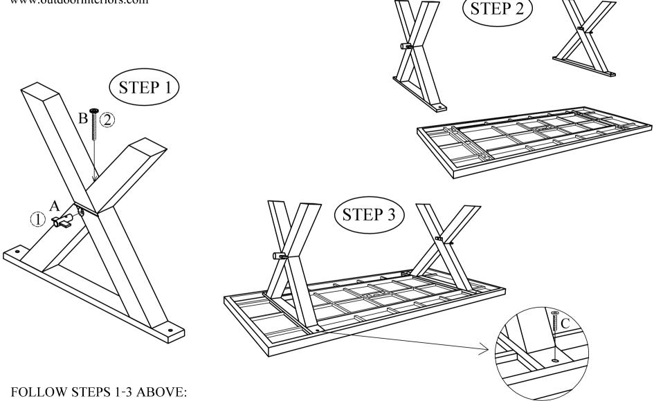
ASSEMBLY TIPS: Use Caution with Heavy Tables and only assemble with a minimum of two people on soft surfaces as not to damage table tops. Assembly should be face down as shown. Use patience when inserting screws & bolts to find the matching holes before locking down to avoid unnecessary damage. Please use care since the Table surface area & parts are handmade. Thanks!
