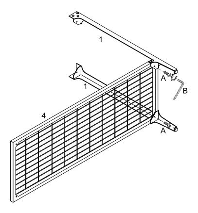
Attach legs (1) to frame (4) using bolts (A) as shown in the diagram.
