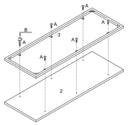
Secure wood panel (2) to frame (3) using bolts (A) as shown.
