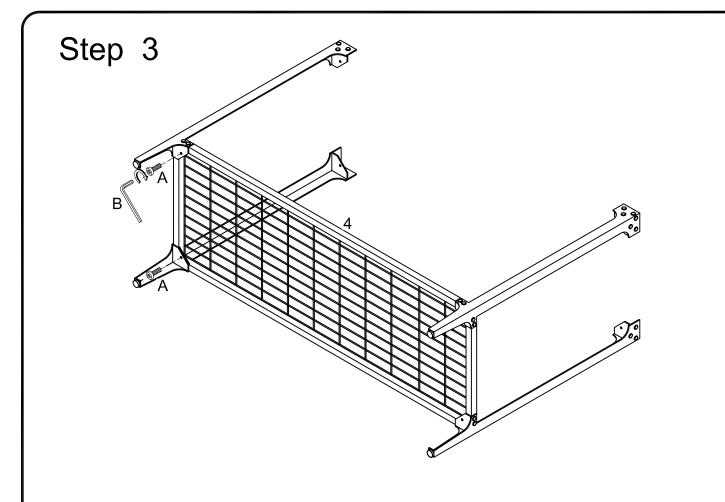
Attach legs (1) to frame (4) using bolts (A) as shown in the diagram.
