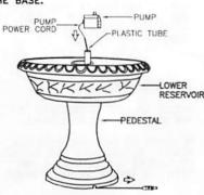
3. PLACE UPPER RESERVOIR ONTO LOWER COLUMN AND TWIST THE UPPER RESERVOIR CLOCKWISE TO SECURE. PLACE UPPER COLUMN INTO UPPER RESERVOIR AND TWIST THE UPPER COLUMN CLOCKWISE TO SECURE. MAKE SURE YOU FEED THE FLEXIBLE HOSE THROUGH THE UPPER RESERVOIR HOLE DOWN TO THE LOWER COLUMN, READY FOR CONNECTION TO PUMP.
