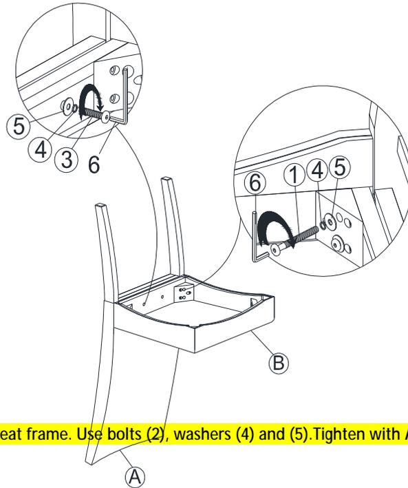
Attach front legs (C) to the seat frame. Use bolts (2), washers (4) and (5). Tighten with Allen Key (6). Attach bottom removed on the step 1 on seat frame.
