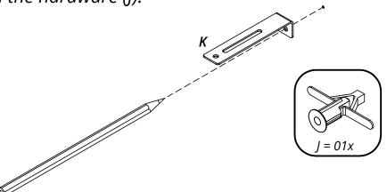
Use the 3/8" drill bit to drill the wall.
