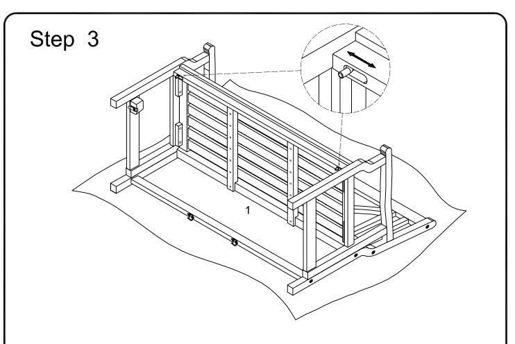
Slide the two locks inward at each end of bench seat, rotate seat up 90 degree until it meets the stops on side legs and push LOCKS OUTWARD TO LOCK into place, Set bench upright.
