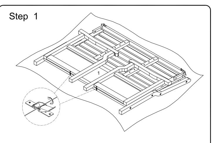
Put bench on a soft working surface, with bench laying flat, unlock at bottom of legs.
