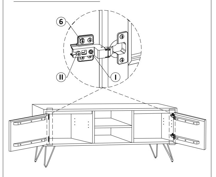
Tighten the Screw marked (II) to fasten hinge. The door may need to be adjusted so that all the spaces between the door and the unit sides are equal. to adjust, follow instructions:
