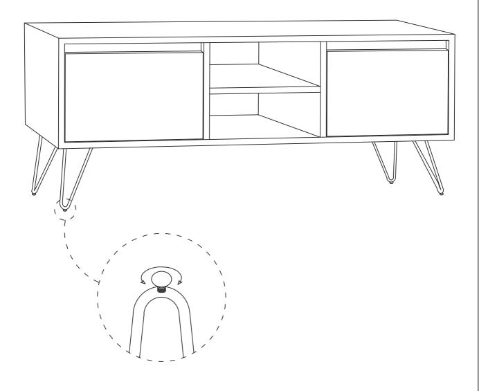
**Note:** Levelers on bottom of legs can be adjusted if floor is uneven.
