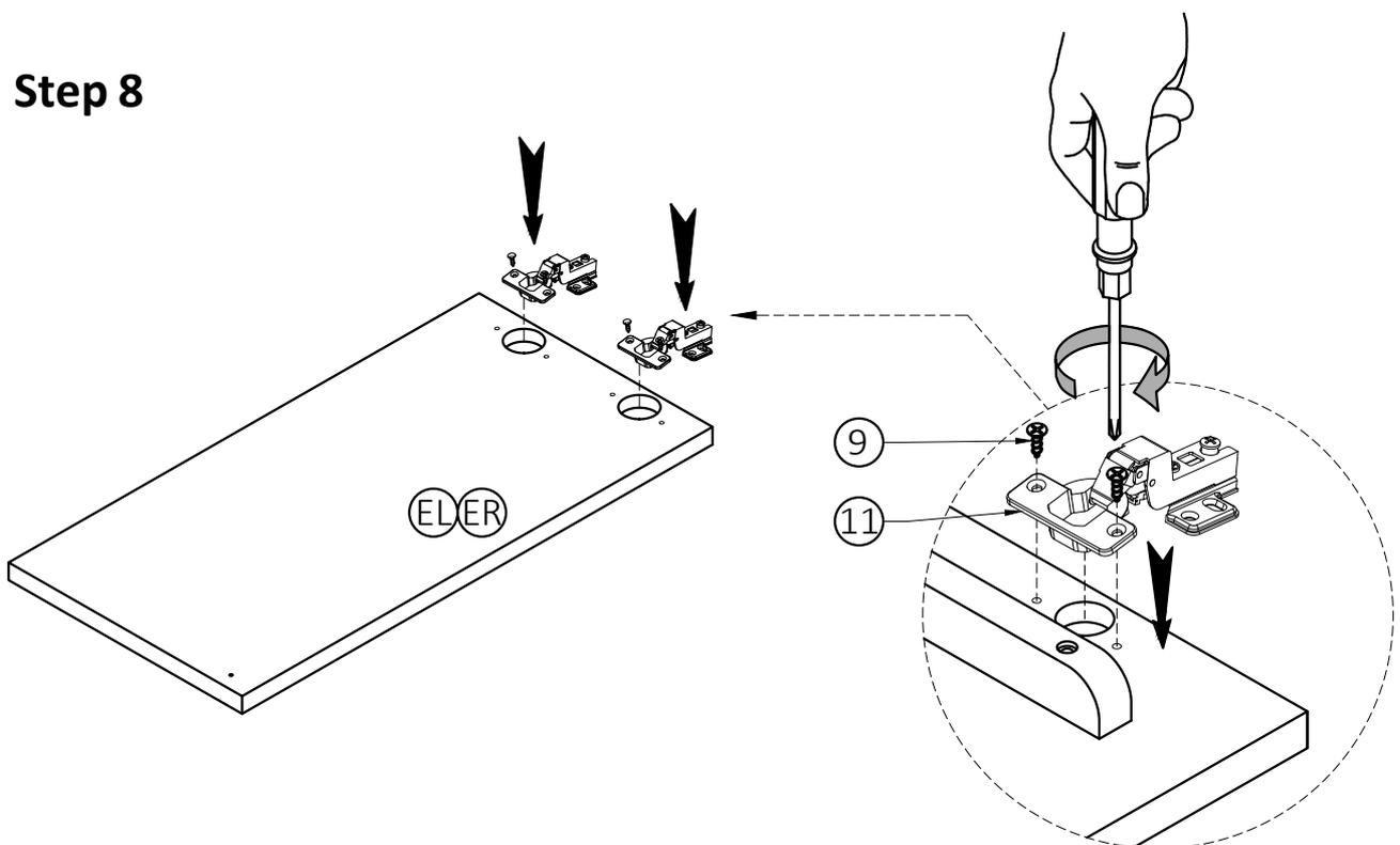
1. Attach Adjustable Hinges (11) to Doors (EL, ER) using Phillips Screws (9) into guide holes on Doors (EL, ER).
