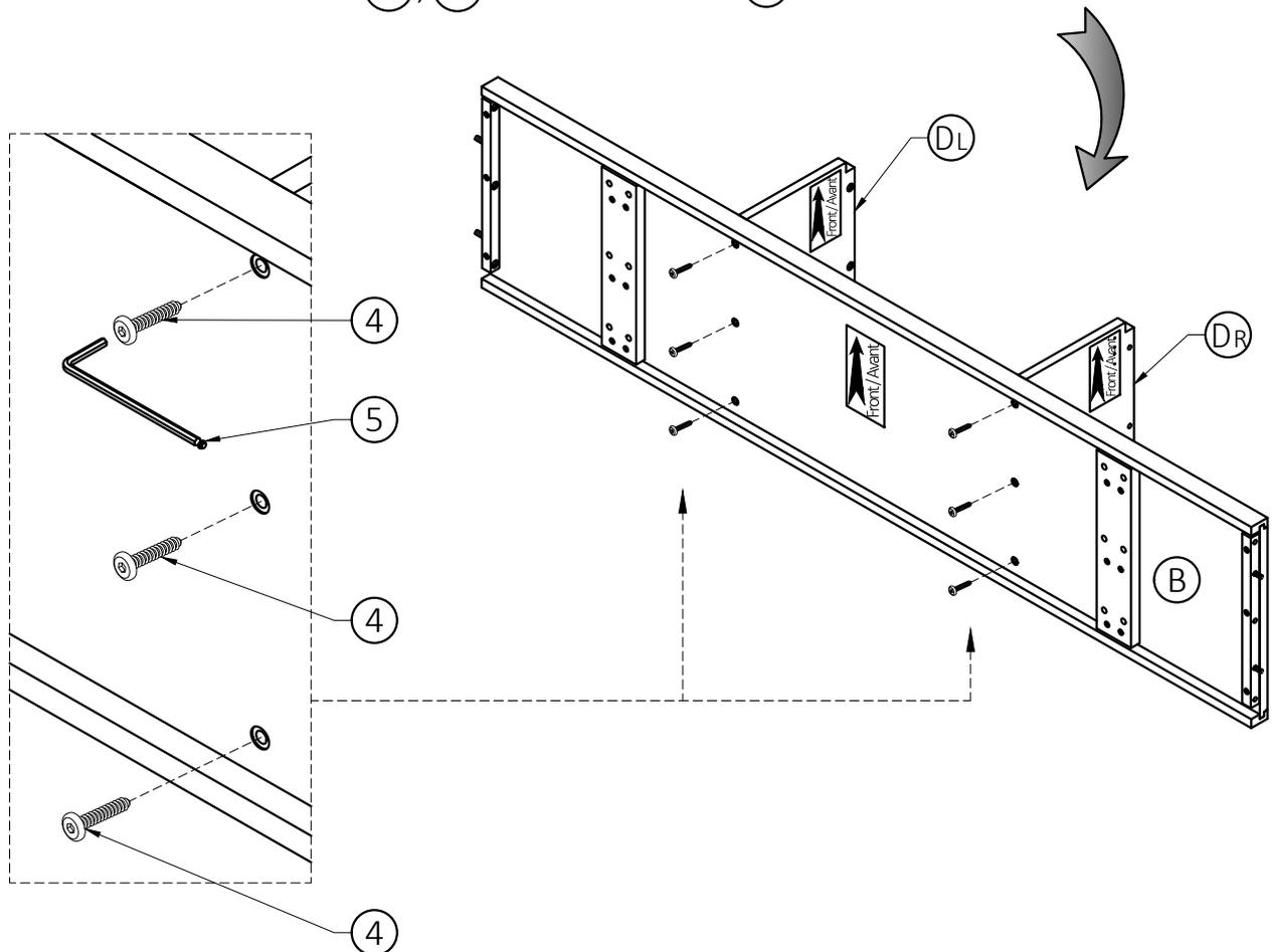
2. Use three Allen Key Screws (4) to attach each Divider (DL), (DR) through guide holes.
