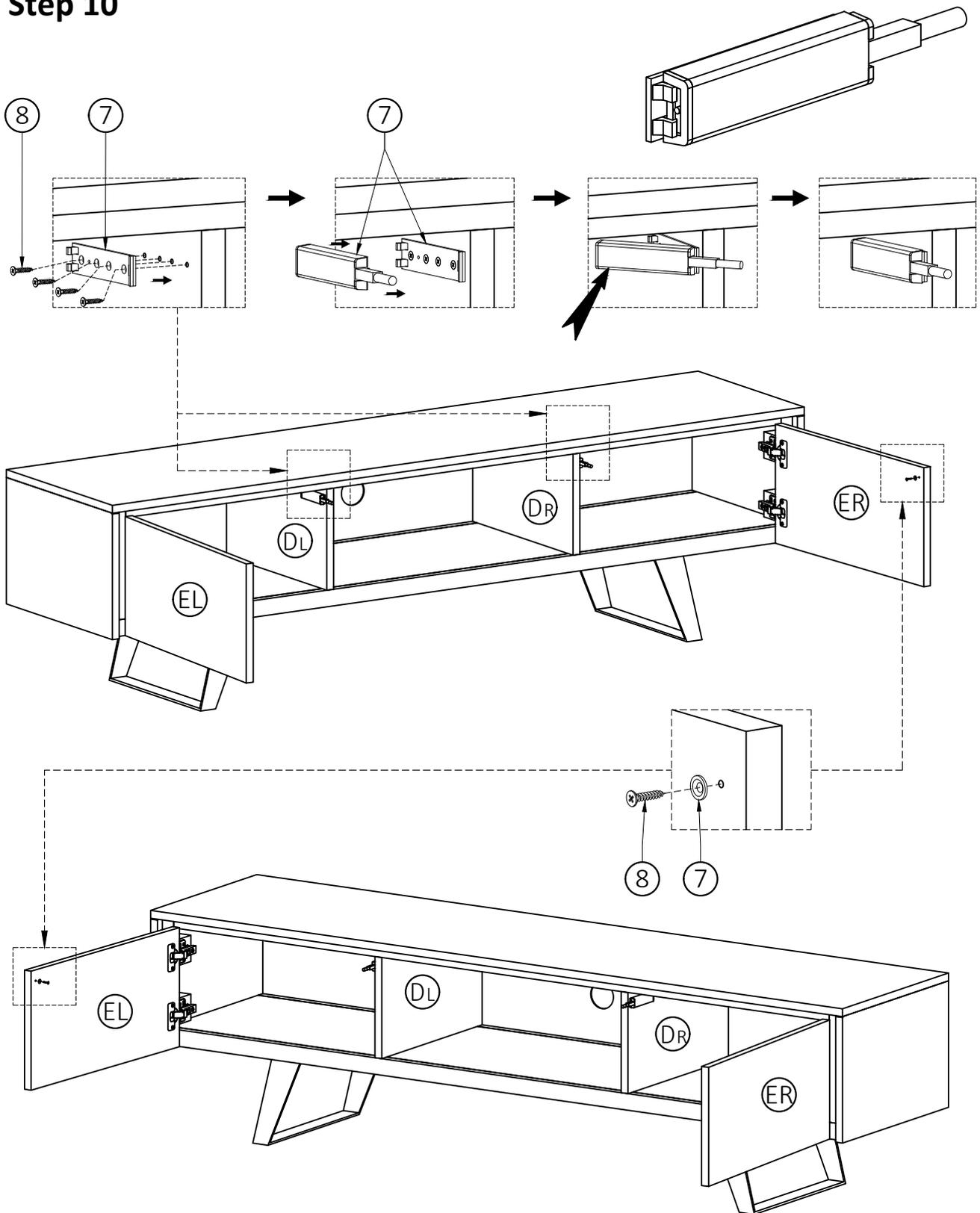
1. Attach Magnets (7) using Phillips Screws (8) into guide holes on Dividers (DL, DR).
