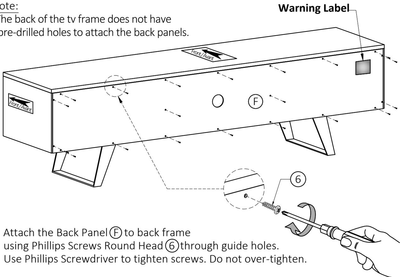
1. Attach the Back Panel (F) to back frame using Phillips Screws Round Head (6) through guide holes.
