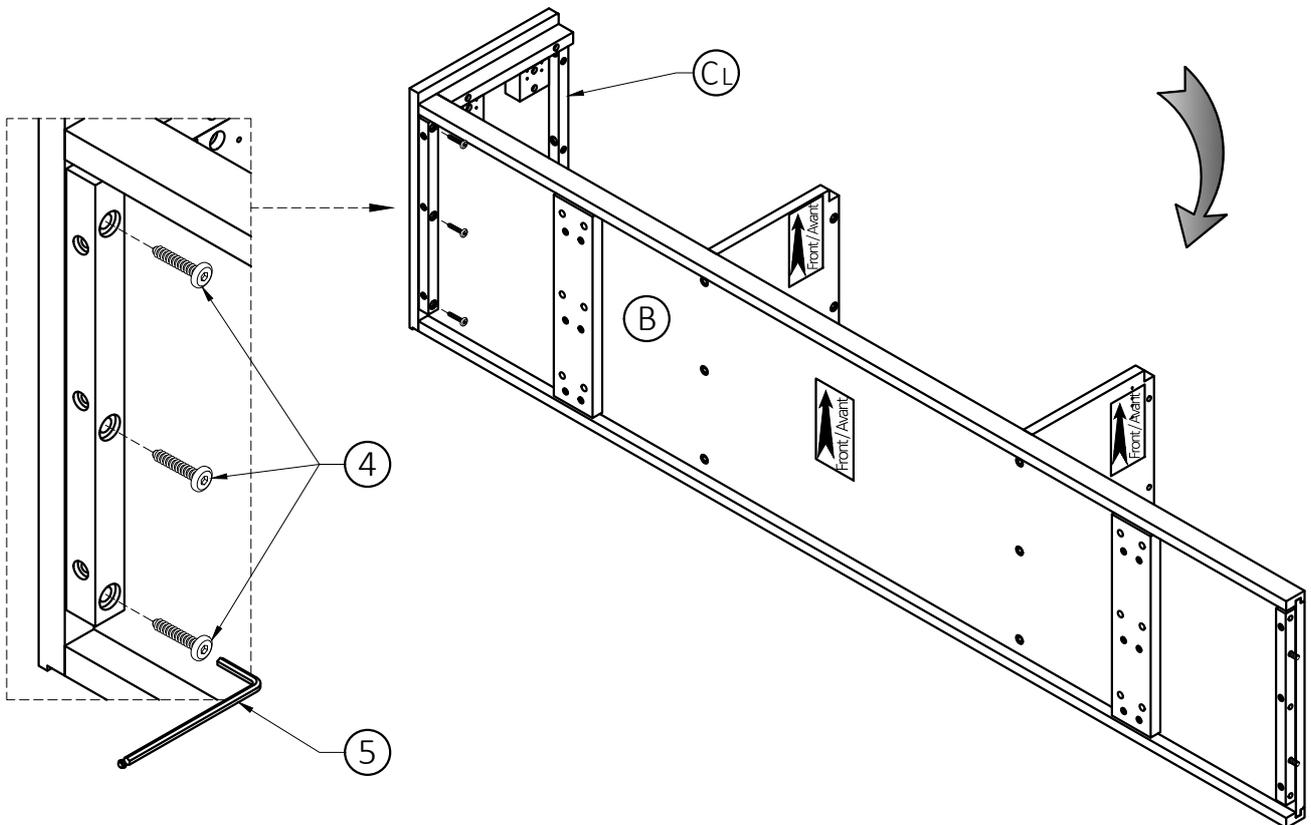
2. Use three Allen Key Screws (4) to attach Left Side (CL) through guide holes.
