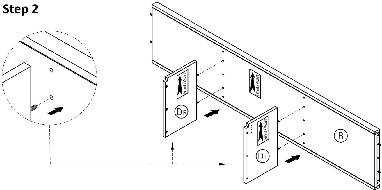
1. Align Wood Dowels with guide holes on each Divider (DL), (DR) and attach each Divider (DL), (DR) to Bottom Shelf (B).
