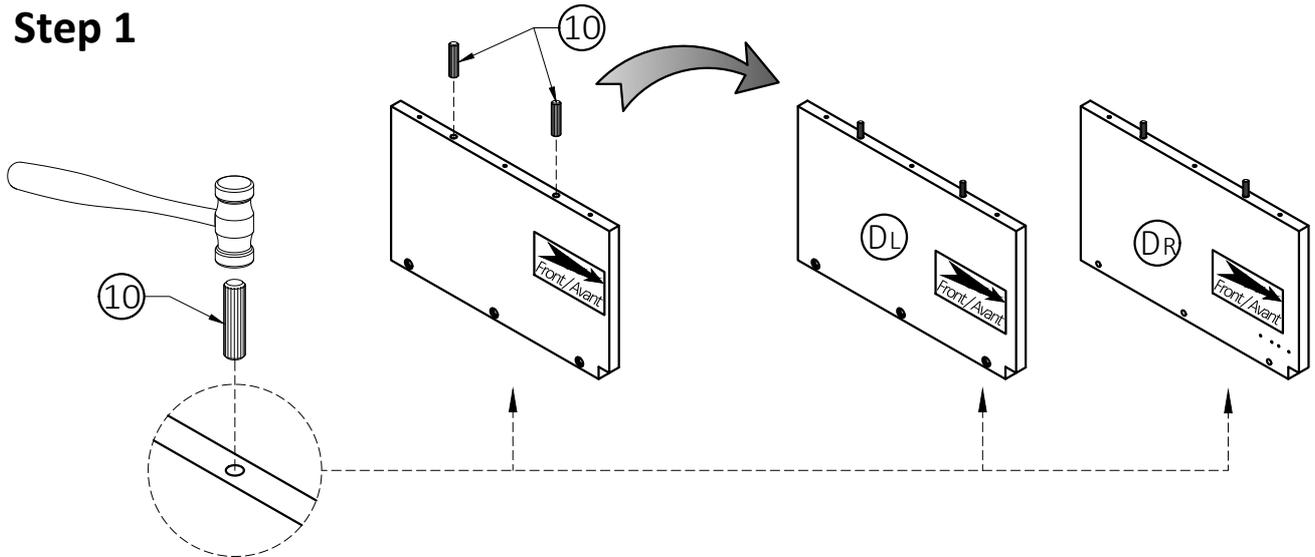
1. Insert two Dowels (10) into drilled holes on each Left Divider (DL) and Right Divider (DR).
