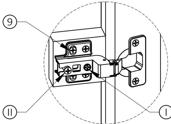
Tighten the Screw marked (II) to fasten hinge. The door may need to be adjusted so that all the spaces between the door and the unit sides are equal. To adjust, follow instructions:
