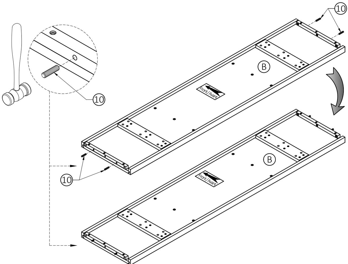
3. Insert four Dowels (10) into drilled holes on Bottom Shelf (B).
