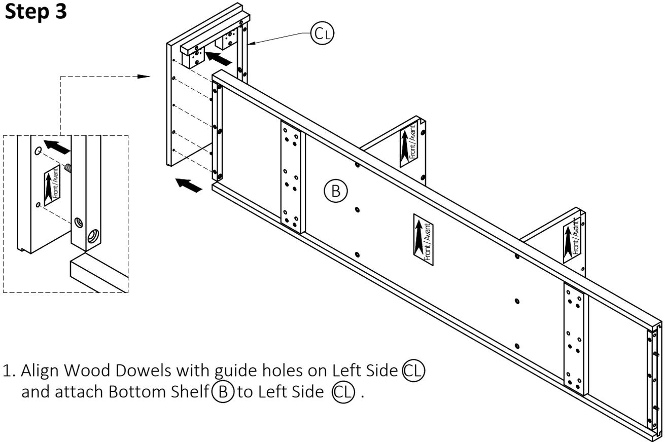
1. Align Wood Dowels with guide holes on Left Side (CL) and attach Bottom Shelf (B) to Left Side (CL) .
