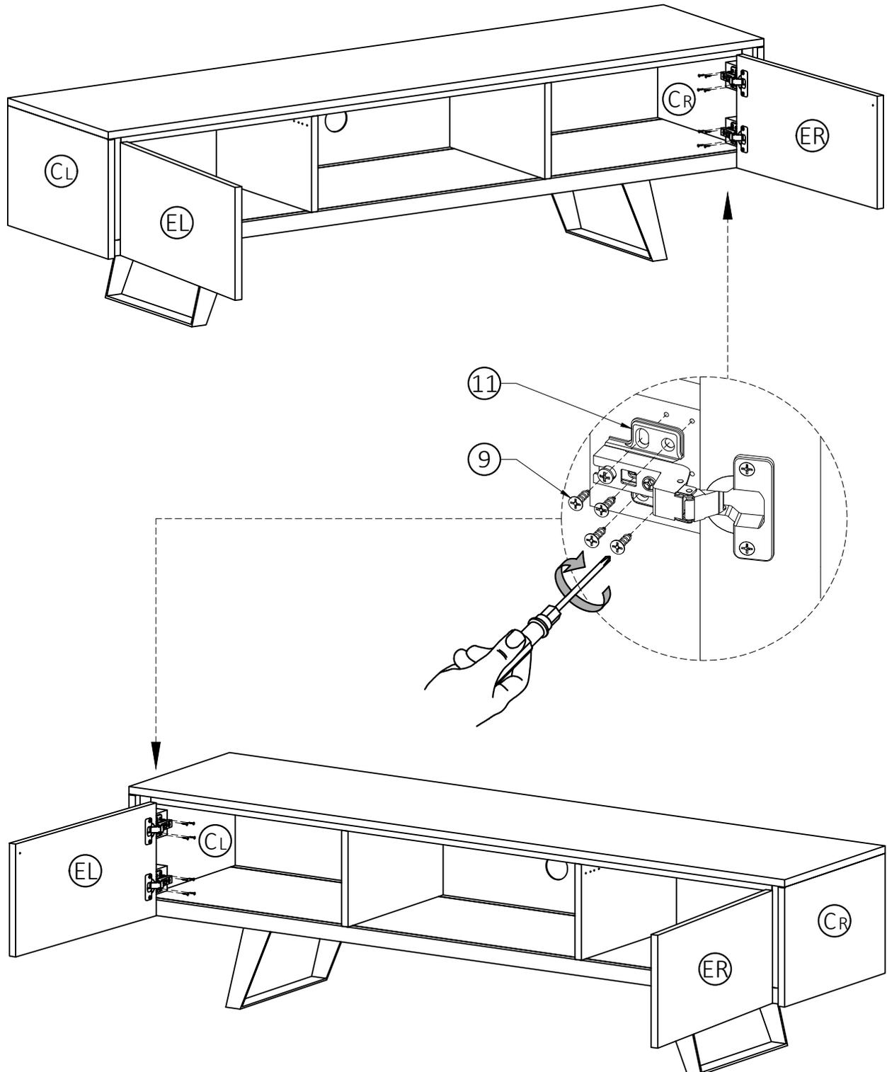
1. Attach Adjustable Hinges (11) on Doors (EL, ER) to Sides (CL, CR) using Phillips Screws (9) into guide holes on Sides (CL, CR).
