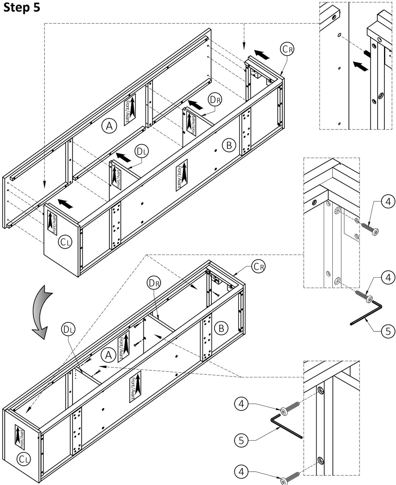
1. Align Wood Dowels with guide holes on Top (A) and attach parts (CL), (CR), (DL), (DR) to Top (A).
