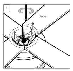
Place motor assembly on a suitable area of Styrofoam and install blades onto motor with set screws provided. Tighten all screws securely.
