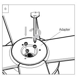
Install an adapter onto the plate on the motor using the set screws removed on last installation step.
