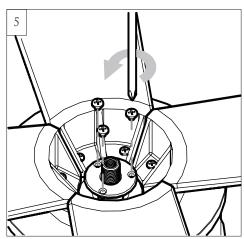
Remove the set screws from the plate on motor. Keep screws
