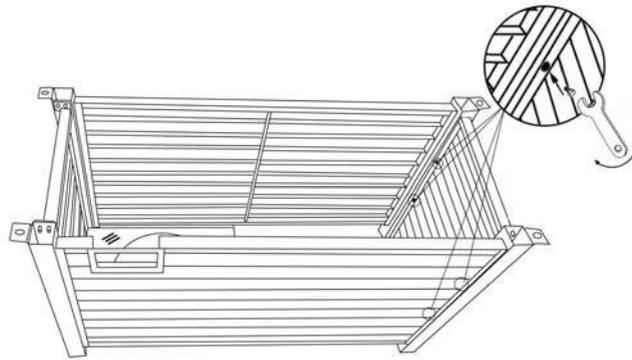
5. Attach Panels (G),(F) and (H) using 4 Screws (e) using the Wrench (d). Fully tighten all screws.
