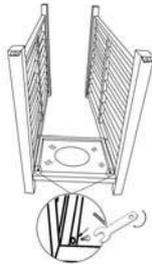
2.Put tank Holder(J) into panel(F) and panel(H). Attach it with 2 screws (a) using the Wrench(d). Please do not fully tighten.
