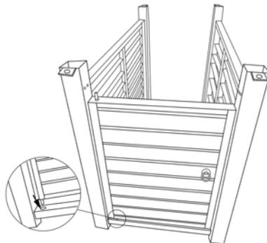
3.Insert Door (I) into the hole on the Tank Holder(J).
