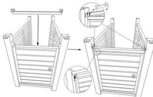
4.Attach the Rail (K) to the Door (I) and Panels (F) and (H) using 4 Screws (e) using the Wrench(d). Please do not fully tighten.
