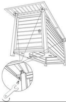
7. Secure the metal base to the Top using 4 Screws (b) and (c) using the Wrench (d).
