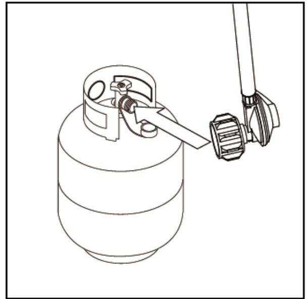
The cylinder used must include a collar to protect the cylinder valve.
