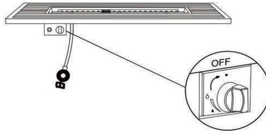
1, Check the control knob for gas supply system is turned to OFF position before starting your assembly.
