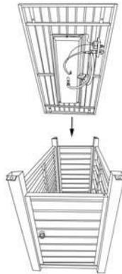
6. Fit the Table (B) onto the metal base, making sure the metal base mates with the window of the Panel.
