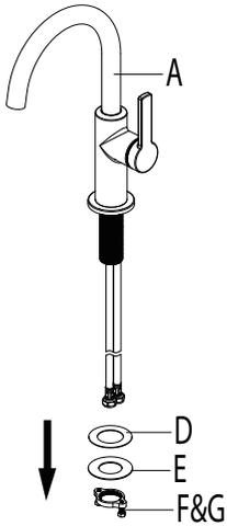
Shut off the water supply. Remove the old faucet. Clean the mounting surface. Remove the mounting nut & screws (F&G), metal washer (E) and plastic washer (D) from the faucet (A).
