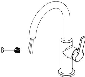
After installing the faucet, remove the aerator (B) with a coin. Turn the water on for 30 seconds to remove any debris. Reassemble the aerator (B).
