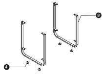
Tighten and Insert Upper Frames (A) into Lower Frames (B) using Bolts(2).
