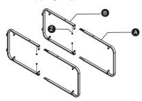
Attach Connecting Bars(C) to the back of Lower Frames
