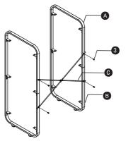
Attach Shelves (D) to Lower Frames (B) and Upper Frames (A) using Bolts(1) as shown below. Note:Do not tighten Bolts(1) until all panels are attached.
