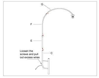
Step 1: Install G, F, E, and C first, and pull out the excess wire in the light pole from the bottom.
