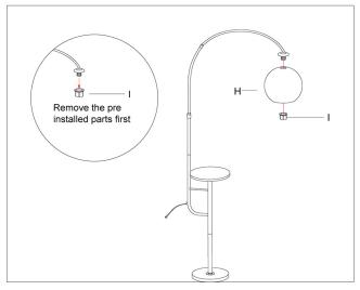
Step 5: Remove the I from G, install H onto G with I. Install a E26 light bulb(not included).
