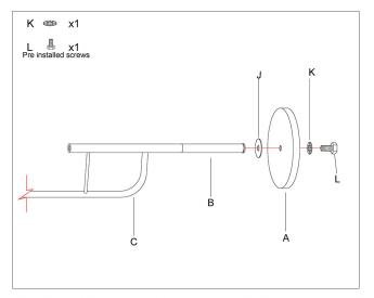
Step 3: Put the assembled G+F+E+C+B flat on the soft pad, pass L through K, A, J in order, and screw in the hole at the bottom of B. Please use a wrench to tighten.
