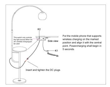
Step 6: Insert and tighten the plugs between D and C, Plug in and switch on the main power by K1, switch on the light by K2.
