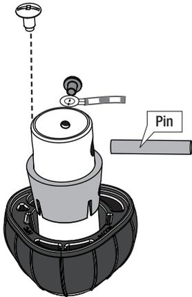
Here is another view of the downrod assembly unassembled.
