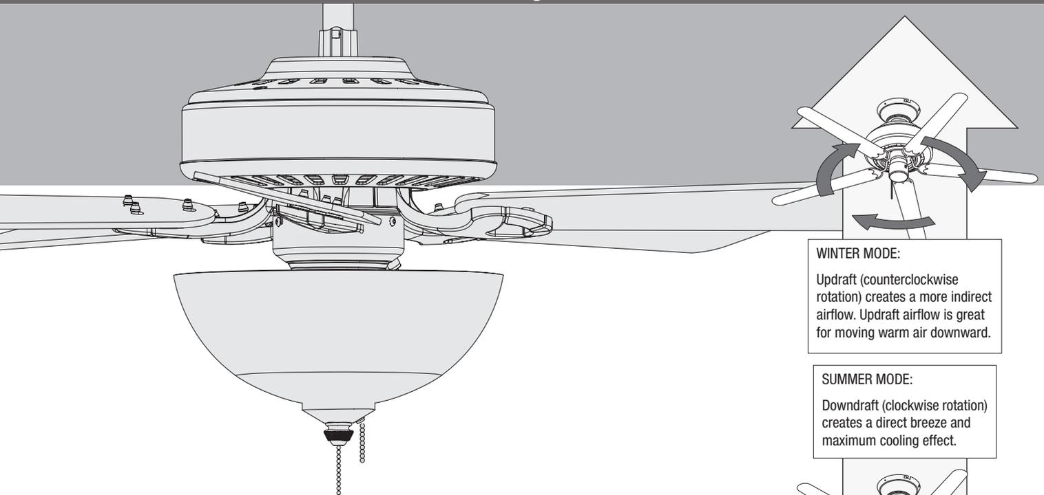
Ceiling fans work in two directions: downdraft (counterclockwise rotation) and updraft (clockwise rotation). To change the fan's rotation direction, wait until the fan comes to a complete stop (audible triple beep). Then pull the fan chain and continue to hold it until you hear a double beep. This beep indicates that the direction has been successfully changed.
