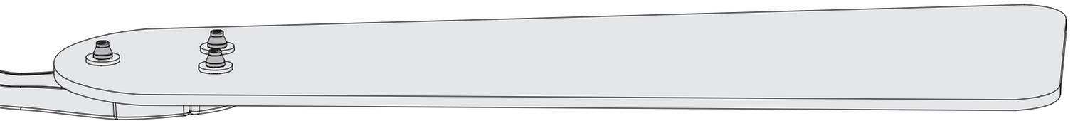
The flared tops of the blade iron posts will be fully visible above the blade when properly assembled.
