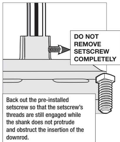
Back out the pre-installed setscrew so that the setscrew's threads are still engaged while the shank does not protrude and obstruct the insertion of the downrod.
