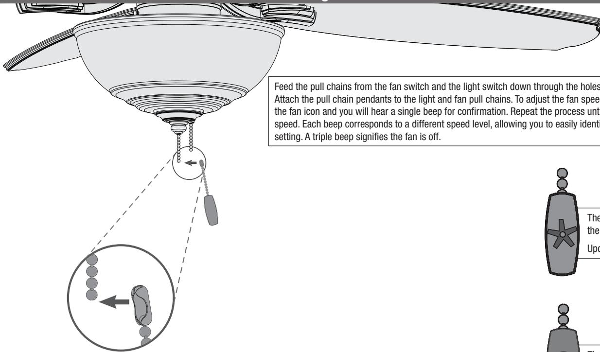
Feed the pull chains from the fan switch and the light switch down through the holes in the finial as shown. Attach the pull chain pendants to the light and fan pull chains. To adjust the fan speed, pull the chain with the fan icon and you will hear a single beep for confirmation. Repeat the process until you reach your desired speed. Each beep corresponds to a different speed level, allowing you to easily identify and select the desired setting. A triple beep signifies the fan is off.
