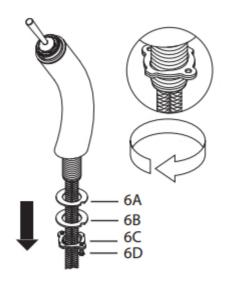
Remove mounting hardware (6A, B, C, & D) from the mounting pipe
