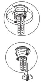
Adjust direction of faucet body (5). Tighten mounting nut (6C) until snug. Tighten mounting screws (6D) to nut with a Phillips head screwdriver until snug
