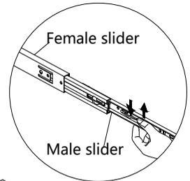
**Schematic diagram of slide rail disassembly**
