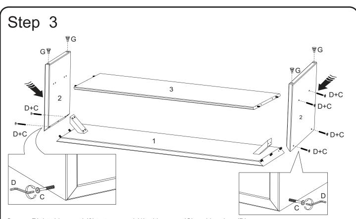
Secure Right side panel (2) to top panel (1) with screw (C) and hex key (D). Secure bottom shelf (3) to side panels (2). Then secure Left side panel (2) to top panel (1) using screw (C) and hex key (D). Insert adjustable Foot (G) Into side Panels (2).
