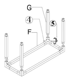
Step 2: Attaching the Top Frame with the Support Poles
