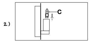
Step.2: Fit the bulbs (C) into each socket. Do not use bare hands to install.
