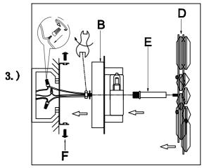
Step.3: Screw the tube(E) on the Crystal lamp frame(D), then lock (E) on the backbox(B) with nut. Connect the wires with the wiring cap
