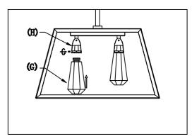
Step 2: Attach crystal (G) to fixture using Allen screws (H) provided.
