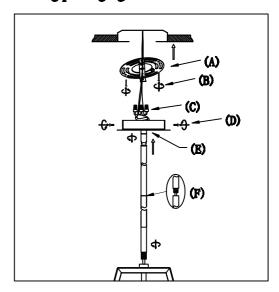
Step 1: Run wire through stems (F) and combine stem lengths to meet desired mounting height. Remove mounting bracket (A) from fixture and install to electrical box. Wire fixture (C) to wires in outlet box. Green wire is Ground wire. Attach the canopy (E) to the mounting bracket using screws (D) on the sides to secure.
