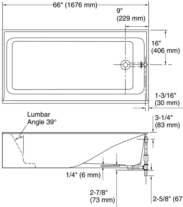
No change in measurement if connected with drain illustrated. (K-7259)
