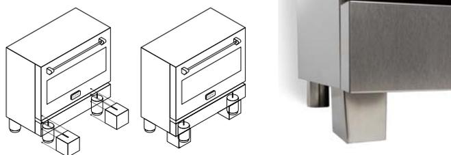
**NOTE:** If the range is not level, the cooking will be uneven. When adjusting the legs, ensure they are the same height.
