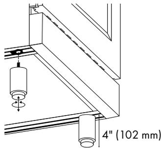
Before installing the legs, position the appliance near its final location, as the legs are not suitable for moving the appliance over long distances.
