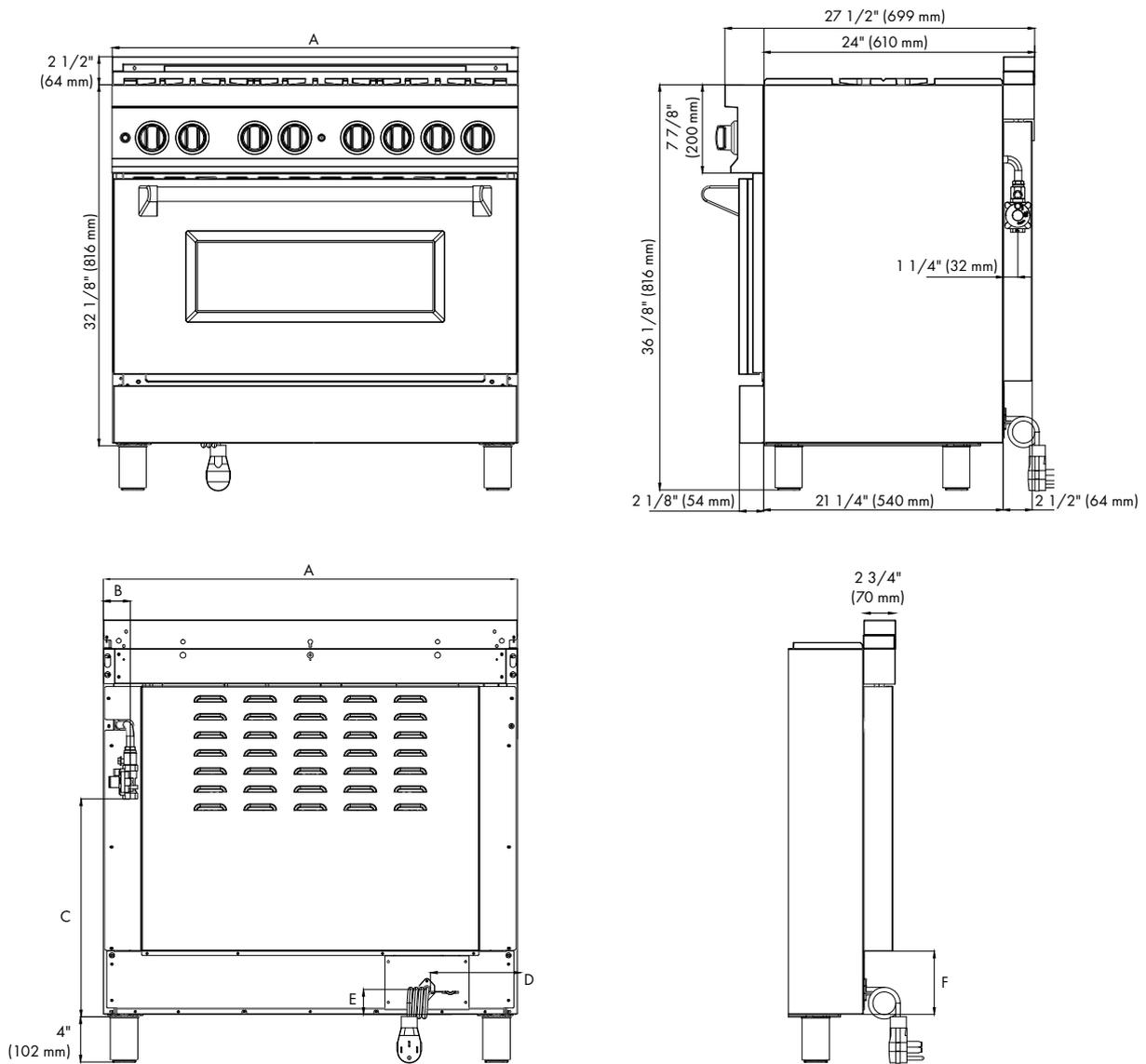
**NOTE:** The above diagram is of the RA36 model; the measurements listed without a letter are universal across all RA models. See the next page for dimensions by model, and for in-depth product and cutout dimensions, see pages 10–11.
