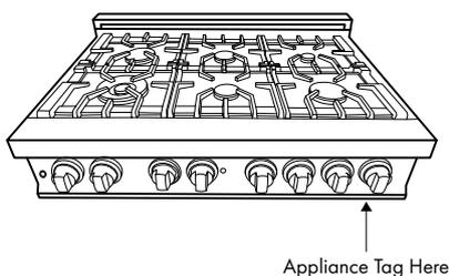
The rating tag shows the model and serial number of your range. The tag is located under the front edge of the range top. The tag is visible when the oven door is open. Do not remove permanently affixed labels, warnings, or plates from the product. This will void the warranty.
