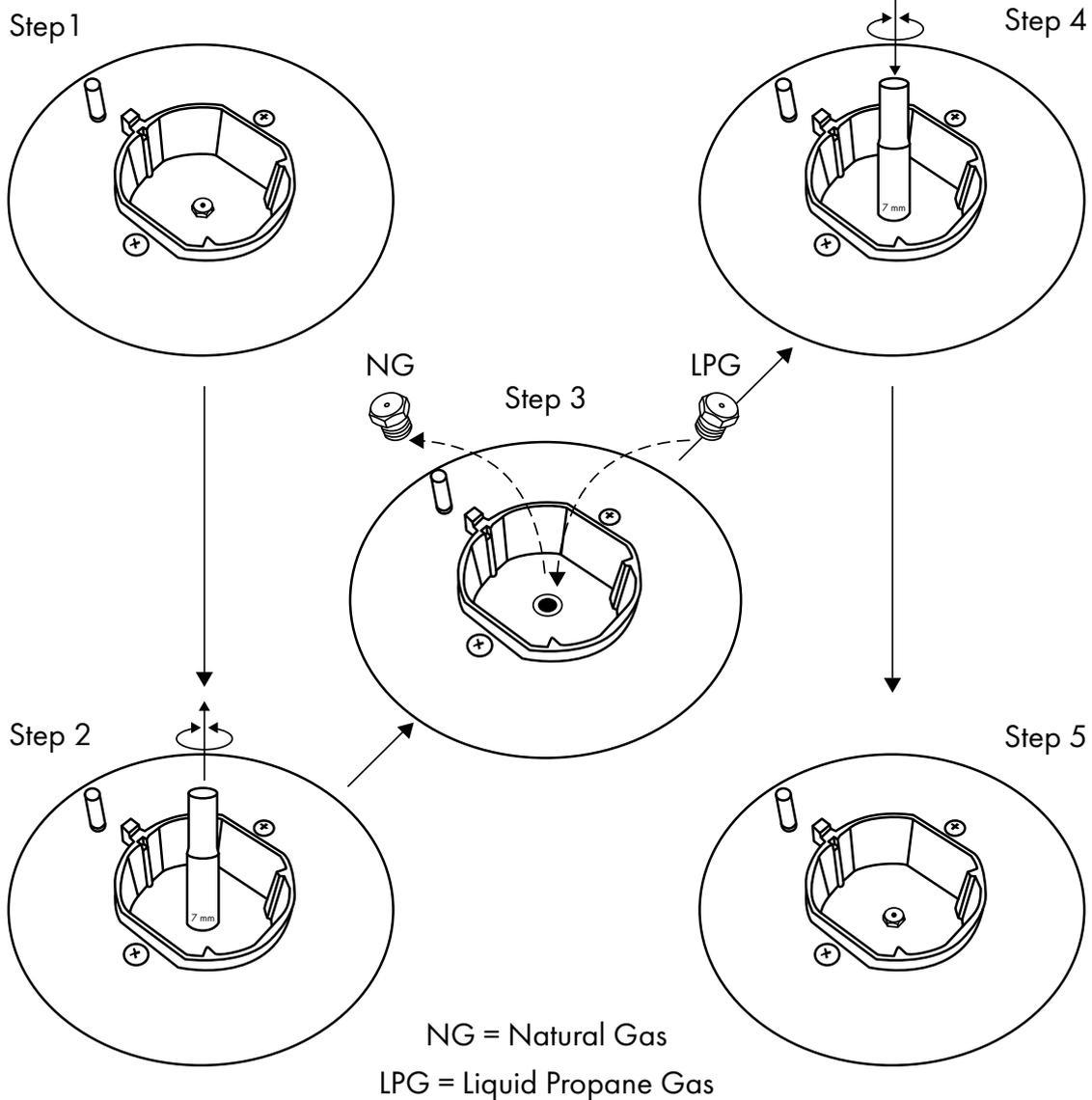
**NOTE:** For the dual burner, the orifice is located on the side of the burner. Use a 7 mm boxed end wrench to remove and tighten.
