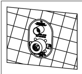
4. Please cut the size of the tile hole according to the size and shape of the protected cover ( about 5mm bigger than the protected cover from each side ) . And please put the tile outside the wooden wall ( please noted that we keep the same central point for the tile hole with the protected cover ) .
