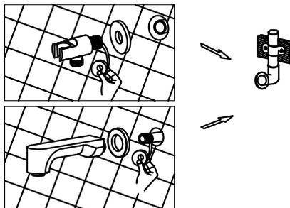
8. Wrap the thread of spout with teflon tape (ensure it must wrap clockwise). Screw-in to the inlet pipe inside the wall, then install the decorative cover on the wall clingy.
