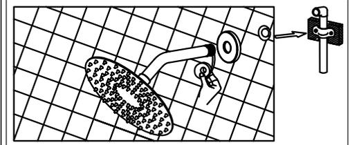
9. Install the shower arm, shower head and flange to the fitting. (stick to the wall) . Tighten the showerhead to the shower arm with the pipe tape. (Make sure the pipe tape with clockwise direction) .
