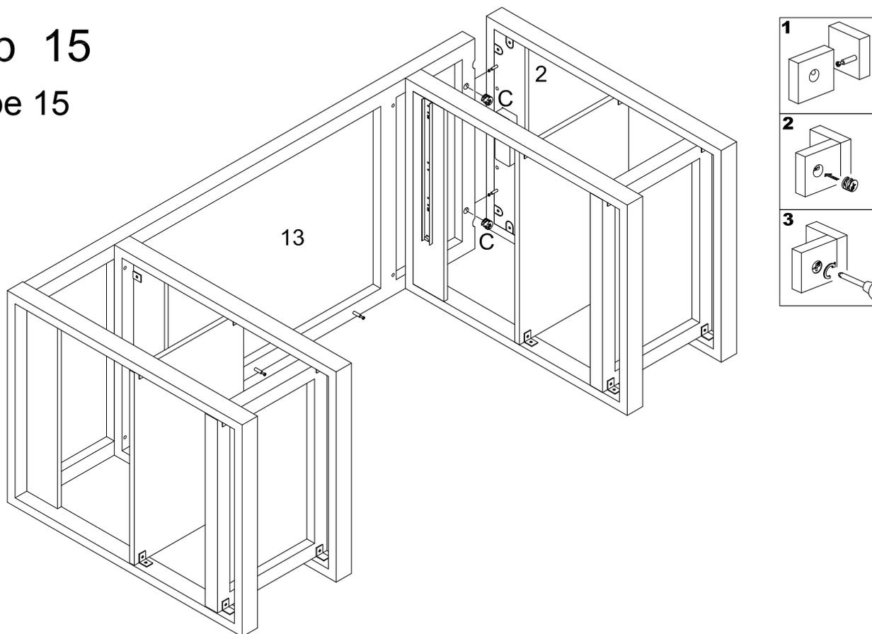
Use cam locks (C) to secure the Table Top (13) to the Side Frame (2).
