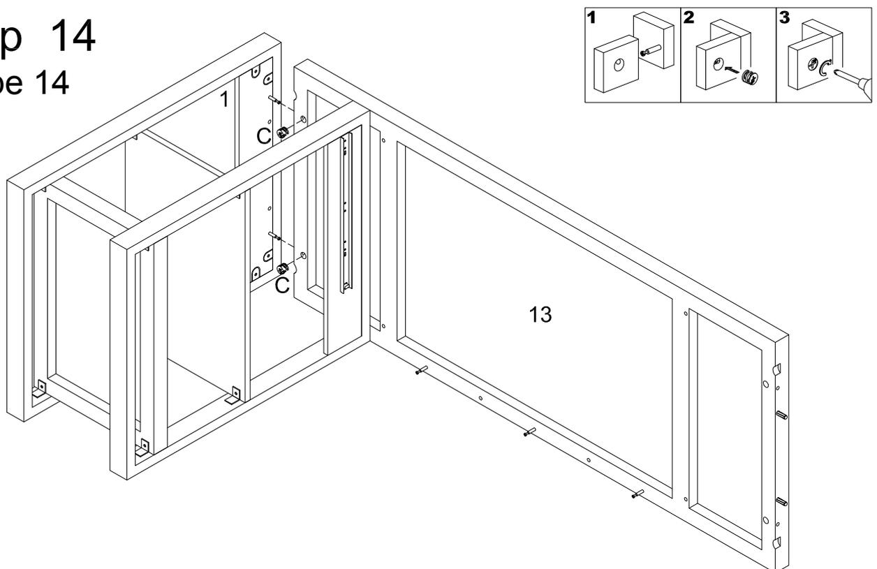
Use cam locks (C) to secure the Table Top (13) to the Side Frame (1).
