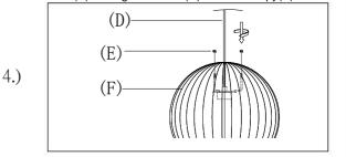
Step.4: Screw in GU24 light bulb and slide canopy back over body.Reattach shade(F) using hexagonal nuts(E).
