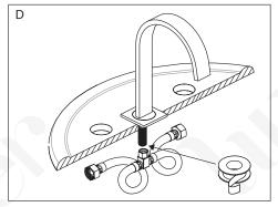
D. Apply Teflon (PTFE) tape on the thread of the center spout brass pipe. Use an adjustable wrench to tighten the fittings. (NOTE: Do not overtighten the connection.)
