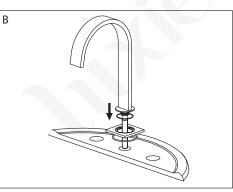
B. Place spout with flange through the center mounting hole on the mounting surface.
