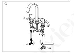
G. Apply Teflon (PTFE) plumbing tape on both valve assemblies and shutoff valves. Attach water supply hoses with 1/2" fittings (not included) with an adjustable wrench. Also connect the water hose between the handle assemblies and the center spout. (NOTE: Do not overtighten the connection.)
