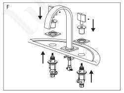
F. Insert hot and cold valves from underneath the mounting surface. Secure the handle assemblies with the decorative trims from top of the mounting surface.
