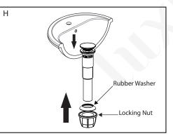
H. Remove rubber washer and locking nut from the drain assembly and slide the drain into the sink. Install the rubber washer first and tighten the locking nut to install the drain.
