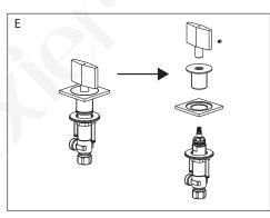
E. Use a small hex wrench to loosen the small setscrew on the handle. Lift up the decorative trim handle and remove all trim pieces.
