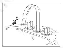
I. Use the aerator wrench to remove the aerator. Turn on both hot and cold handles and let the water run for about 1 minute to flush out any sediment or debris inside the plumbing. Also check for leaks at all connections. Re-install the aerator to complete the installation.
