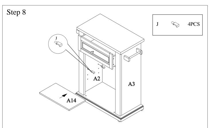
Insert Shelf Supports J into Side Panels A2 & A3, then put Adjustable Shelf A14 onto Shelf Supports J.
