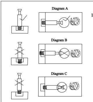
1. Insert cam screw into hole as shown in diagram A.
