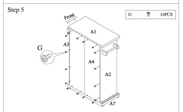
Assemble Back Panel A4 to Side Panels A2 & A3, Top Panel A1 and Bottom Panel A7 using Screws G.
