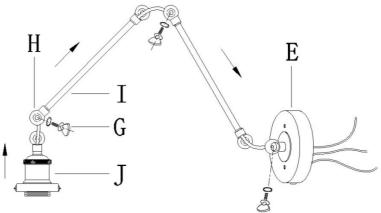
3) Connect the black and white wires found in the plate (E) to the wires with plug found inside the accessories bag. Secure the connections with plastic wire connectors.
