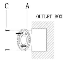
4) Fix the ground copper wire found in plate (E) around the ground green screw (B) found on plate (A) then connect it to its adjacent copper ground wire found in the outlet box. Secure the connection with plastic wire connector (D).
