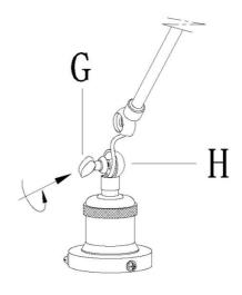
2) Carefully and gently pull the wires and fiberglass sleeve from the another end of arm(I), meanwhile push the socket (J) till two parts of joint are close each other, lay wires in the cave of joint(H), then proceed to push till the two parts are put together, secure with the stud
