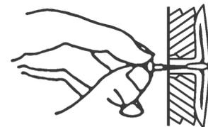
Fig. 19a - Attaching Wall Hanging Spacers to Heater
