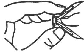
Fig. 18 - Popping Open Anchor Wing For Thin Walls
