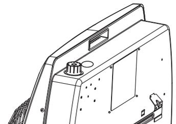
Fig. 10 - Attaching Fan
