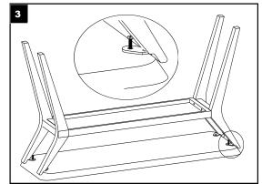
Step 3: use 4 bolt M8x20 ( H2 ) and washer to connect wooden frame and concrete top at metal connecting plate
