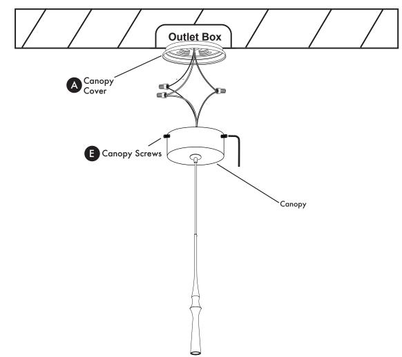
Attach canopy to canopy cover (A). Secure with canopy screws (E).
