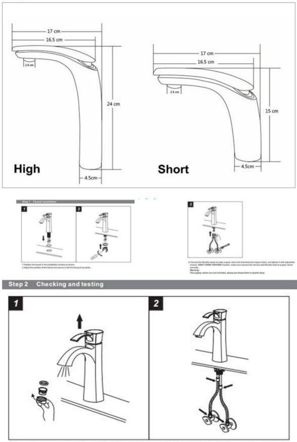
1.Remove the aerator by hand. Turn the faucet handle all the way on, turn on hot and cold water supply and flush water lines for one minute. Reinstall aerator by hand. 2.Check all connections at arrows for leaks, re-tighten it if necessary. BUT DON'T OVERTIGHTEN!
