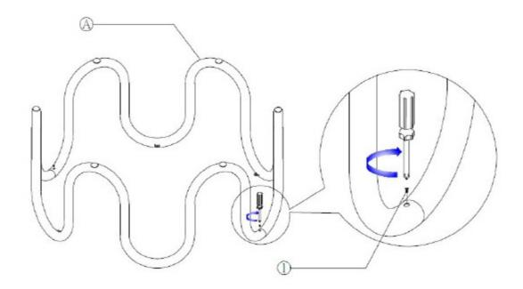
4. Put the assembled Table bases (A) upside down on the Table Top (B), align the pre-drilled holes, secure with the spring washers ④, flat washers ③ and bolts ② using the enclosed Allen Key ⑤.
