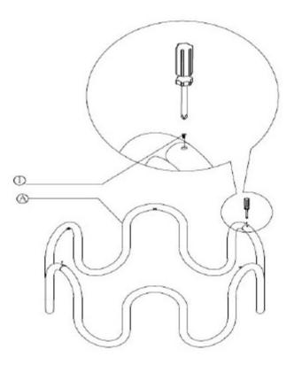
3. Place the assembled Table bases (A) upside down, secure with the Screws ① using the screwdriver on both sides, then need to tighten all screws ① in this step.
