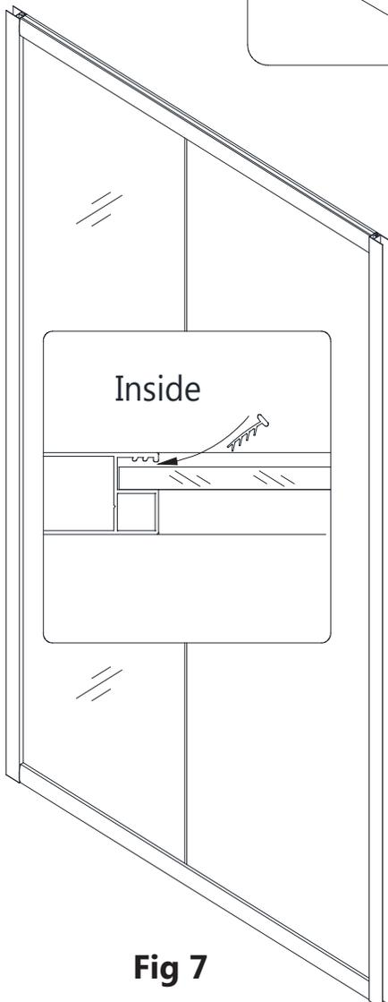
6. Starting from the bottom, insert the **Single Side Strip (#08)** into the groove between the glass and the glass profile using a wooden or plastic shim. The strip should be inserted from the side that will face inside the shower.
