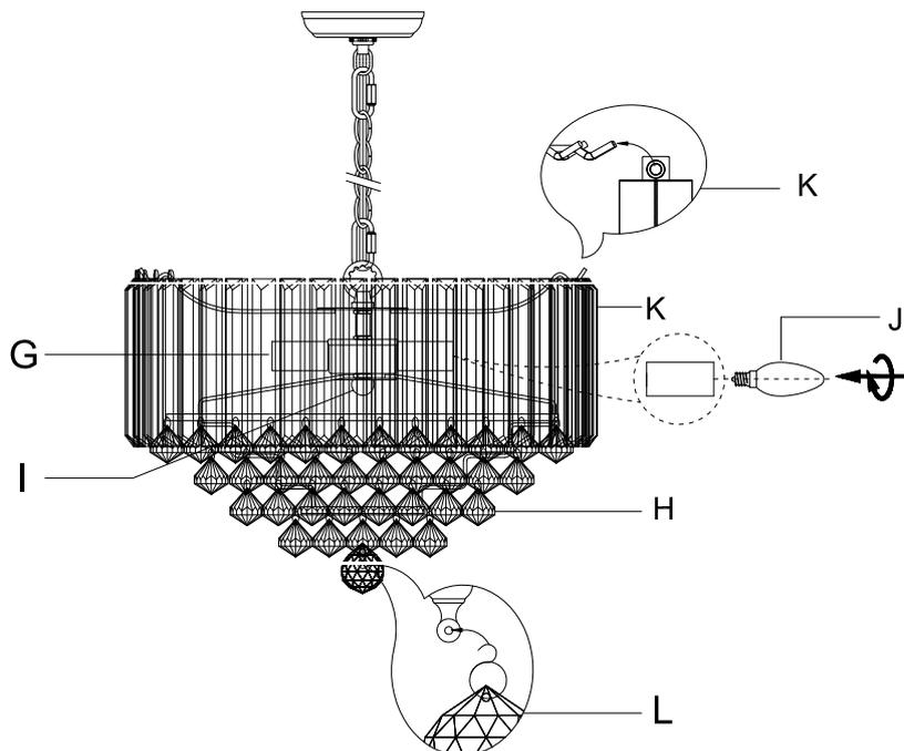
**PLEASE USE TYPE "B" BULB MAX 40-WATT OR CFL BULB MAX 13-WATT OR LED MAX 9-WATT
