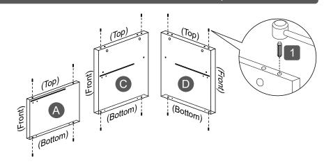
THEN: Install the stoppers #7 to panels A, C and D positioned as shown.
