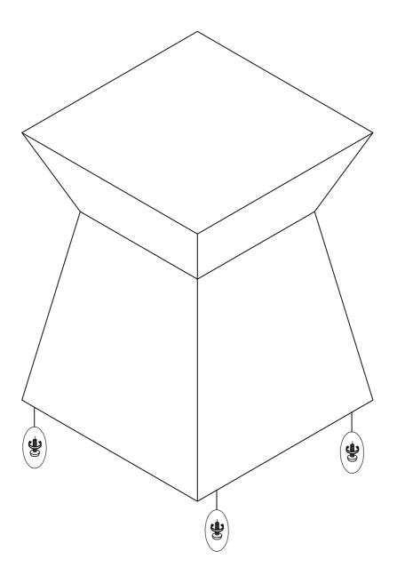
Adjust levelers if needed, to level case on uneven floor
