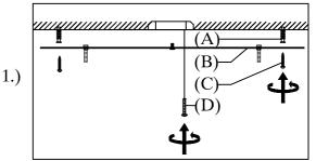
Step1:Remove mounting bracket from fixture and install to electrical box. The safety button mounted to the bracket.
