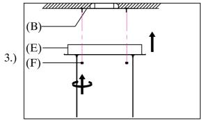
Step3: Install fixture to bracket and Decorative Nuts at the ends of the canopy to secure.
