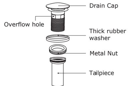
**Step 3:** From under the drain, insert the thick rubber washer and screw on and tighten the metal nut. Remove excess plumbers' putty
