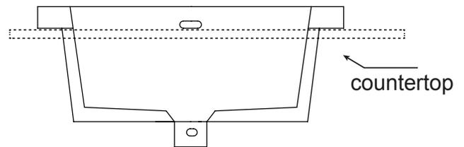
**Step 2:** Place a generous portion of plumbers' putty under drain cap and insert whole drain body inside the bowl and through the countertop.
