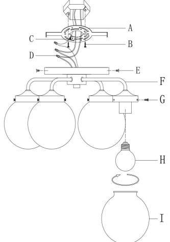
PLEASE USE ON/OFF TYPE"A" BULB MAX 40-WATT OR LED BULB MAX 9 -WATT THERE ARE LED 4PCS 4WATT BULB IN THE BOX
