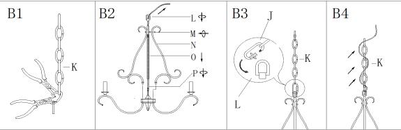
Step B1: By measuring, determine the correct number of links needed for proper hanging height. Using the chain pliers, disconnect and discard the remaining chain.
