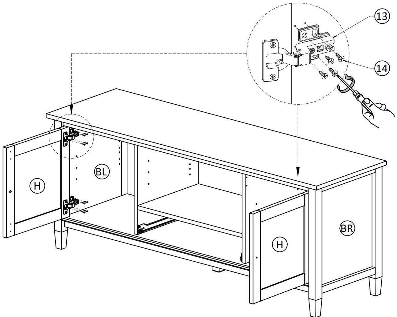
2. Attach Adjustable Hinges (13) on Doors (H) to parts (BL), (BR) using Phillips Screws (14) into pre-drilled holes on Sides (BL), (BR).
