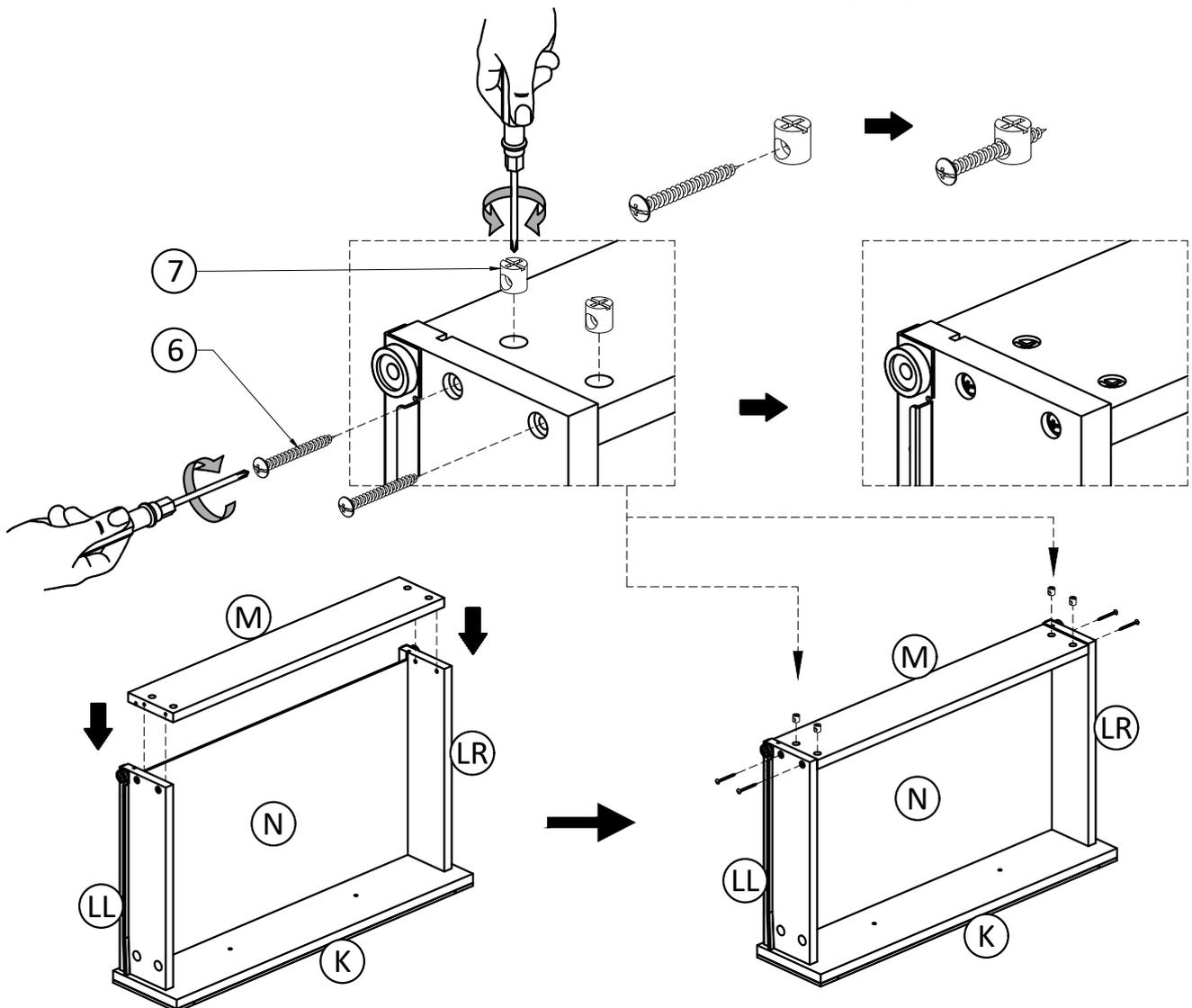
2. Align Drawer Back (M) with Drawer Bottom (N) and press firmly into slot.
