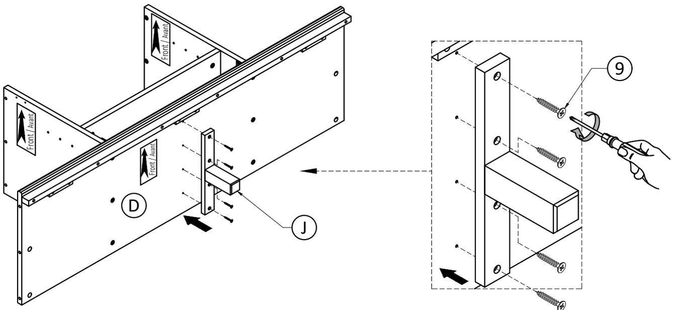
3. Align Bottom Support Leg (J) with pre-drilled holes on back of Bottom Shelf (D). Use Phillips Screwdriver to tighten four Phillips Screws (9).
