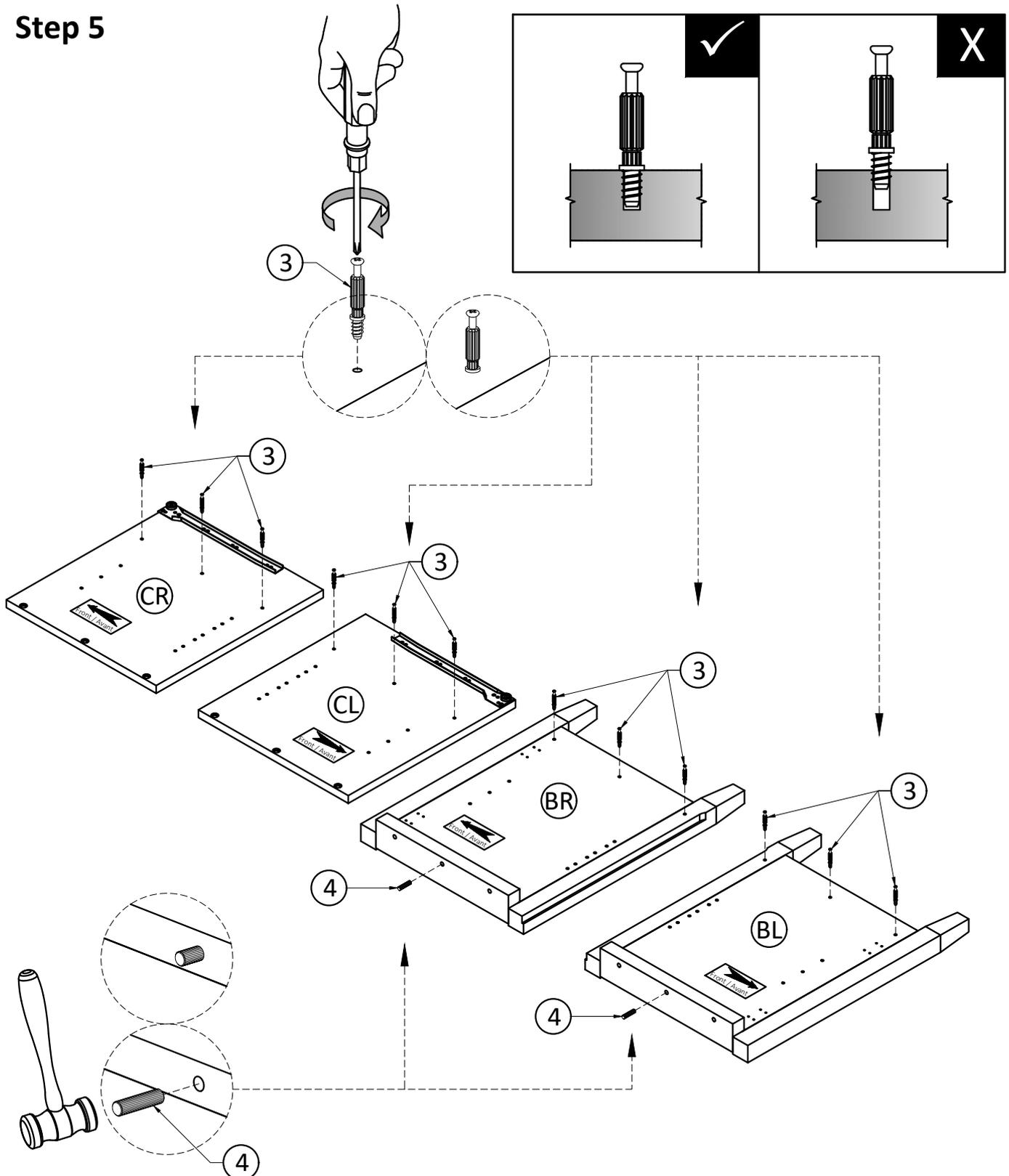
1. Attach three Cam Lock Pins (3) into pre-drilled holes on each Side (BL), (BR) and Divider (CL), (CR).
