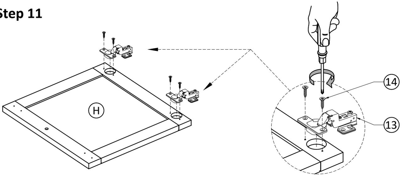
1. Attach Adjustable Hinges (13) to Doors (H) using Phillips Screws (14) into pre-drilled holes on Doors (H).
