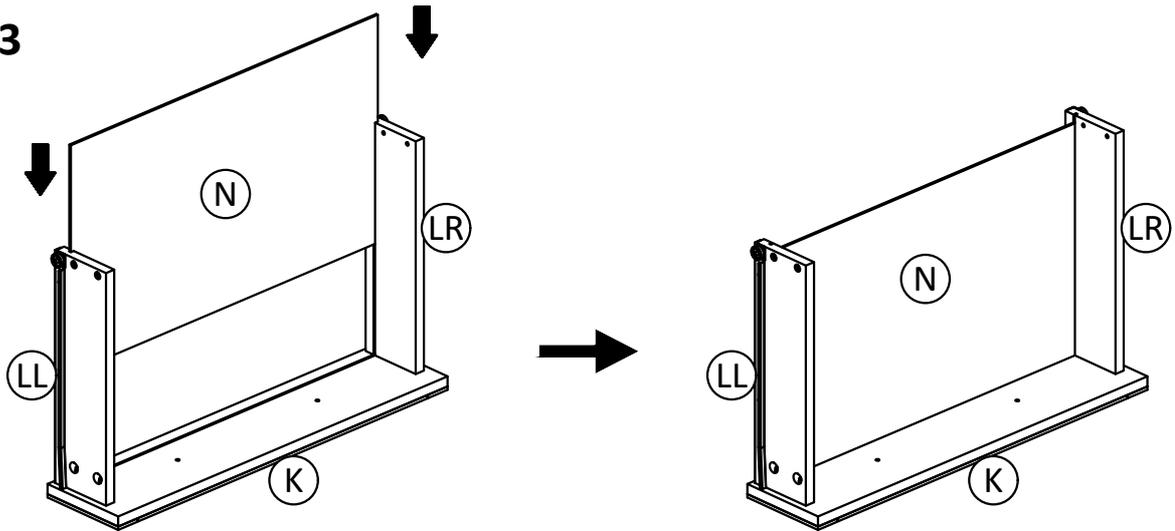
1. Slide Drawer Bottom (N) firmly into slots on Drawer Sides (LL, LR) and Drawer Front (K).
