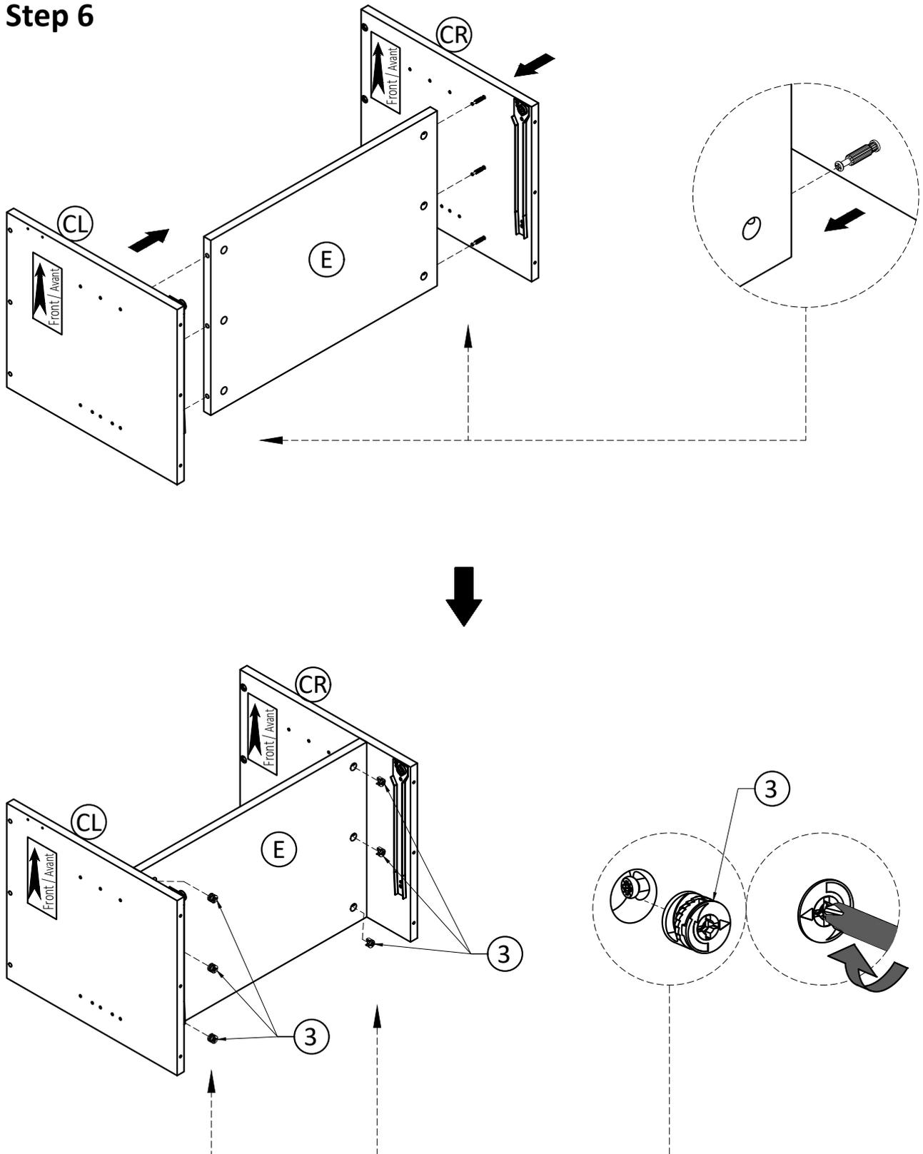
1. Align Cam Lock Pins with guide holes and attach Centre Shelf (E) to Dividers (CL), (CR).
