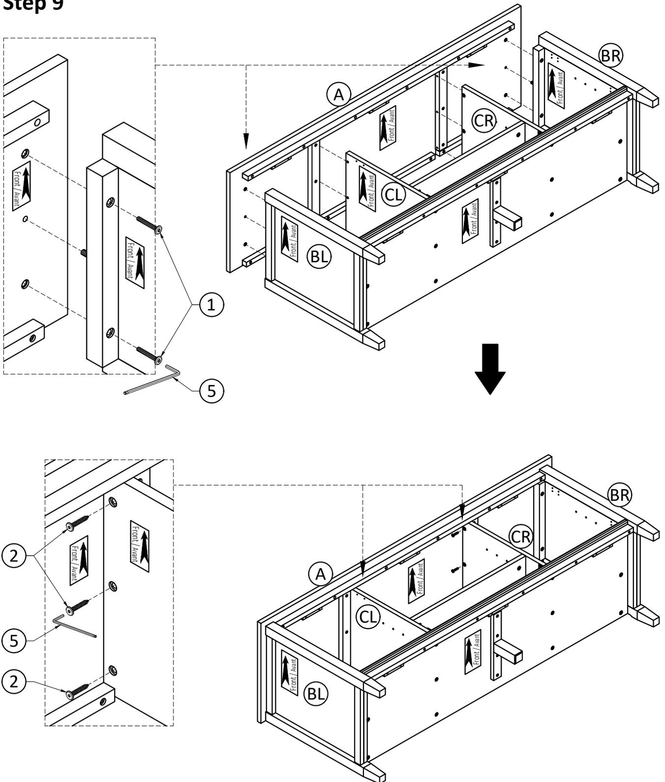
1. Align Wood Dowels with guide holes and attach Top (A) to Sides (BL), (BR).
