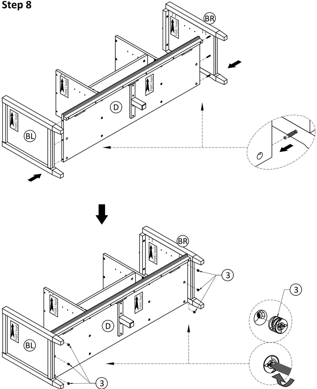
1. Align Cam Lock Pins with guide holes and attach Sides (BL), (BR) to Bottom Shelf (D).
