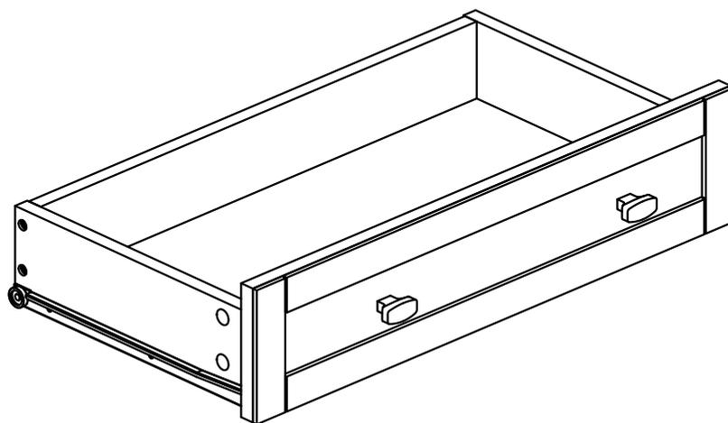
1. Use Phillips screwdriver to attach Handles (8) to Drawer Front (K).
