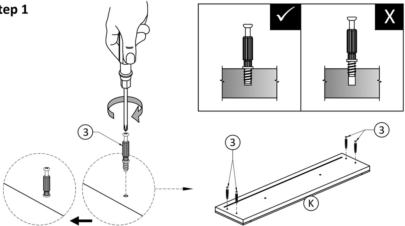
1. Attach four Cam Lock Pins (3) into pre-drilled holes on back of Drawer Front (K).
