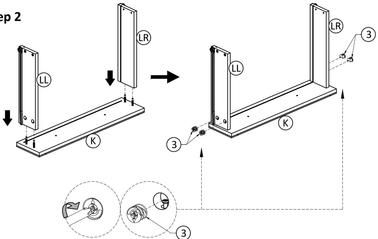
1. Align Cam Lock Pins with guide holes and attach Drawer Sides (LL, LR).
