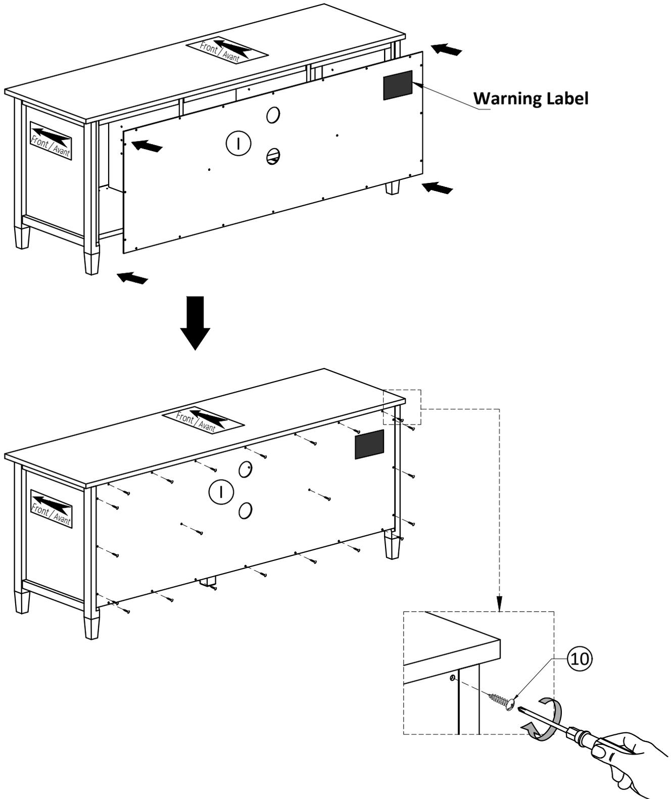
1. Attach Back Panel ① to back frame by using Phillips Screws Round Head ⑩.
