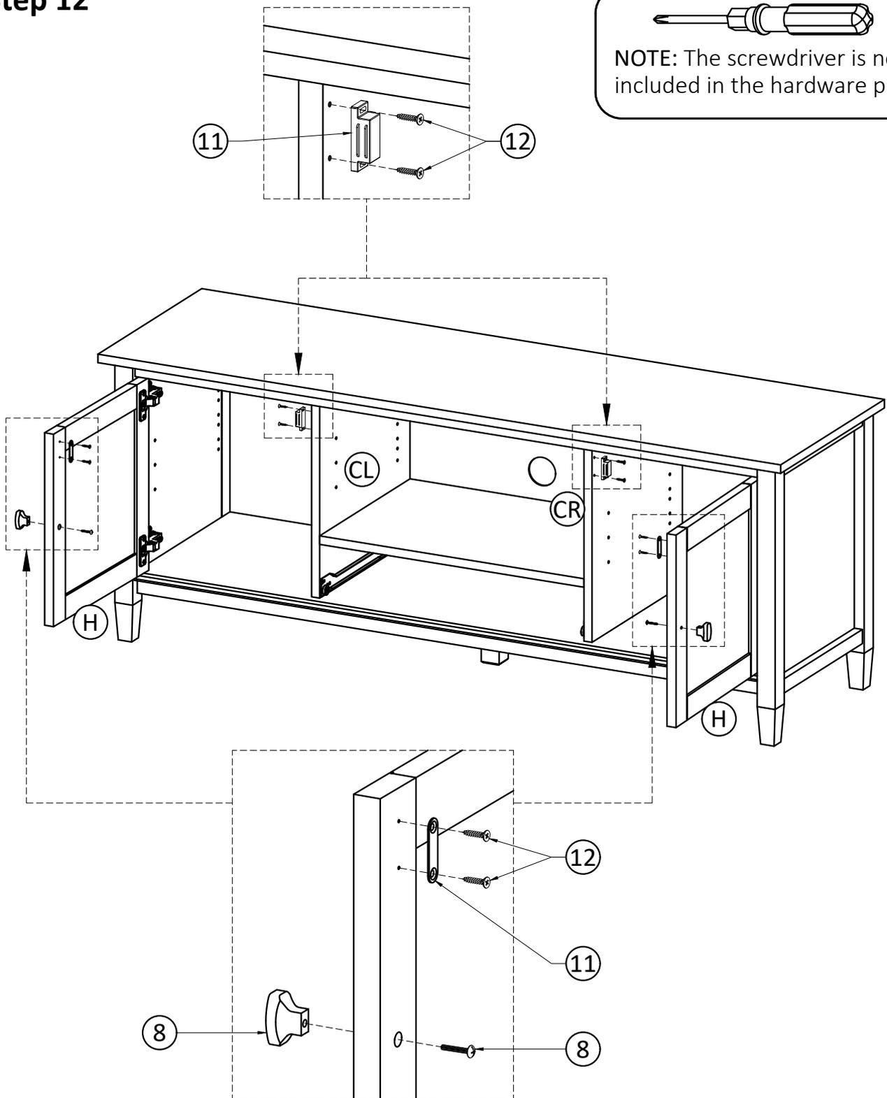
1. Attach Magnets (11) to Dividers (CL), (CR) using Phillips Screws (12) into pre-drilled holes on Dividers (CL), (CR).
