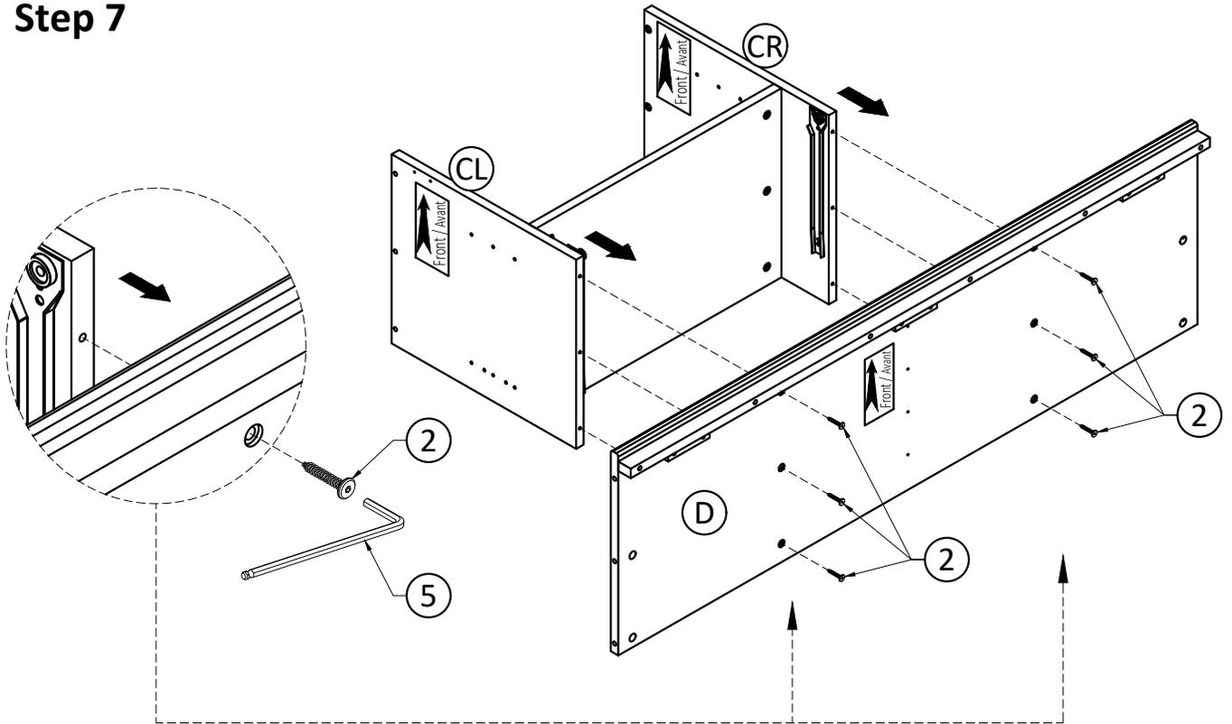
1. Attach Dividers (CL), (CR) to Bottom Shelf (D) using six Allen Key Screws (2) through guide holes.
