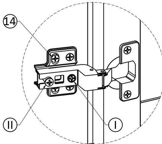
Tighten the Screw marked (II) to fasten hinge. The door may need to be adjusted so that all the spaces between the door and the unit sides are equal. To adjust, follow instructions:
