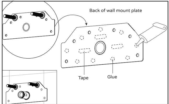
Apply glue (18) to wall mount plate(5) as indicated and add tape (included) to secure onto wall. Place wall mount plate (5) over holes drawn to make sure everything is leveled. Let glue (18) cure for 48 hours for complete result.
