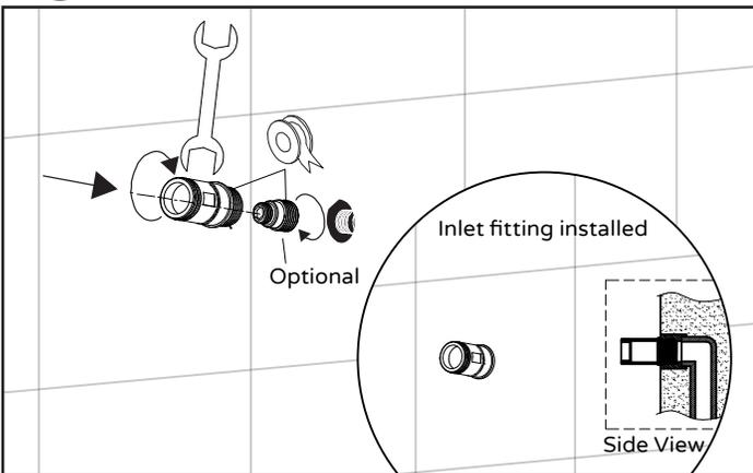
Apply plumber's tape on inlet fitting(4). If you need to use a nipple extension, be sure to also apply plumber's tape. Insert inlet fitting(4) onto existing water supply. Use wrench to secure.
