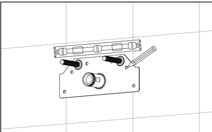
Place wall mount plate(5) over the inlet fitting(4) and make sure it is leveled. Mark holes with pencil.
