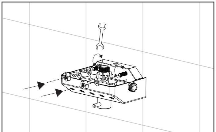
Slide shower body(11) over wall mount plate(5) screws and secure with nut(12).
