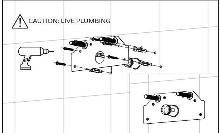
Drill hole previously marked and add anchors(7). Place wall mount plate(5) over the holes and secure with screws(8).
