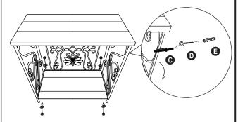
2.Drill holes slightly smaller than anchors (E) into drywall and gently tap anchors into holes.3.Insert eyelet screws (D)to anchors and fasten unit to wall using cable ties (C) .
